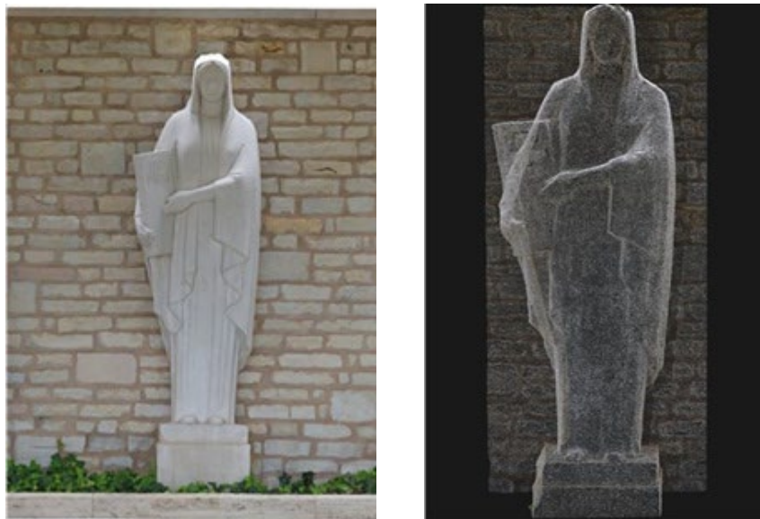
Figure 7. Example of a statue as a textured mesh (left) and a dense point cloud (right).
