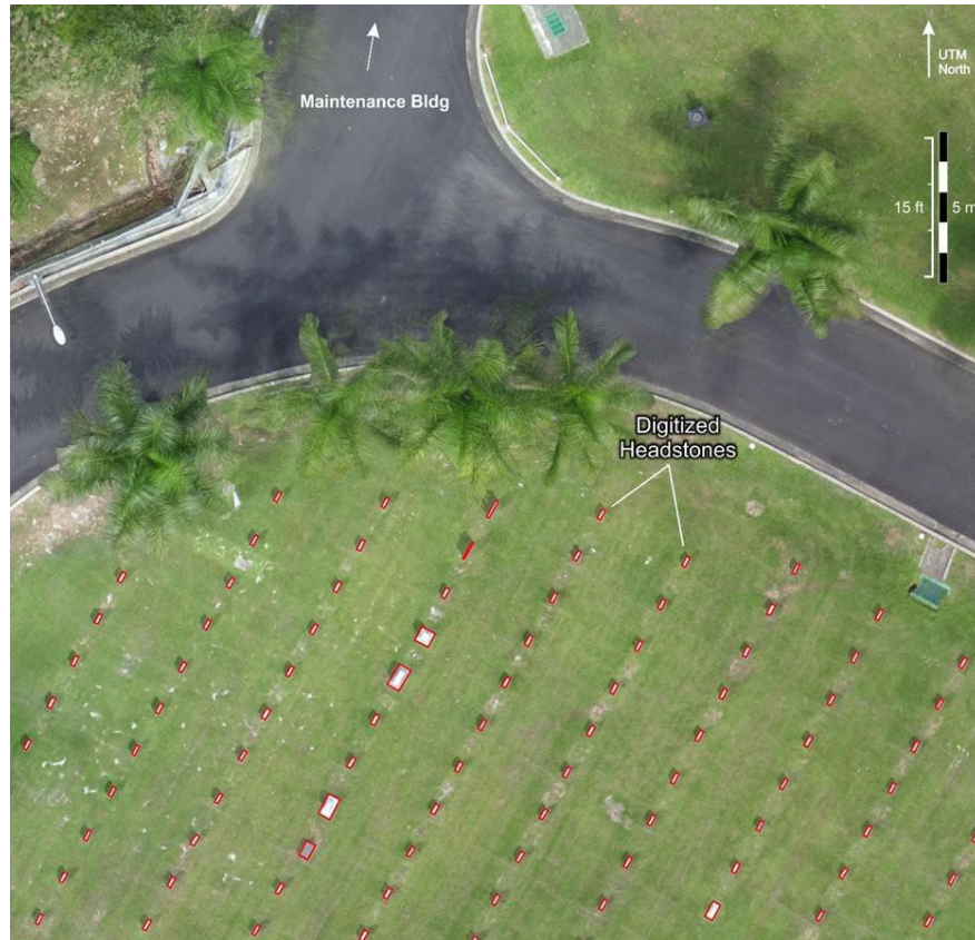
Figure 13. Using the orthophoto-mosaic to vectorize headstone location and size/shape in a large cemetery.
