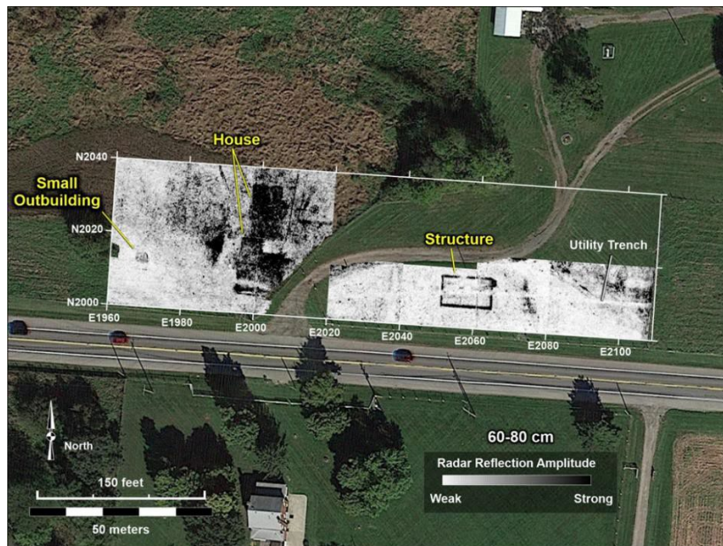
Figure 12. Radar amplitude slice map from 60-80 cm below surface showing building foundations and a modern-era utility line that has cut through them.
