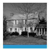
Dense bushes growing close to a building's foundation hold water and keep sunlight from drying the foundation, leading to basement dampness. The bushes pictured here have since been removed from this Lowell, Ohio, home. Every building should be inspected at least twice yearly and more often if problems are evident. Inspections are conducted from the roof down to the ground to follow the path of precipitation and reveal any signs of dampness or damage.
